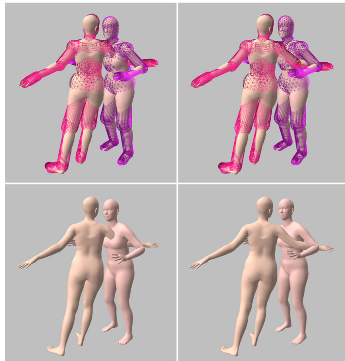
Fig. 4. Without physics-based simulation, avatars may interpenetrate each other in disturbing ways, as shown on the left. With the physics-based simulation in FLSH, on the other hand, interactions are much more accurate, as shown on the right. This example uses the articulated skeleton model. For fast collision detection, each avatar is represented with proxy geometry formed by a hierarchy of analytical capsules (shown in the top images).
