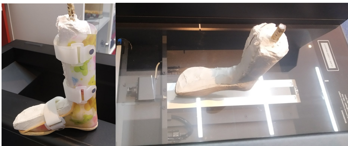
Fig. 3. A plaster positive of the foot is obtained in the correct position, which is then scanned on a 3D scanner
