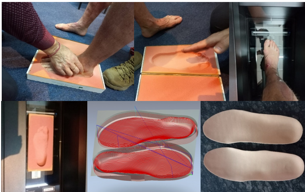
Fig. 12. The Process of Developing Special Inserts to Improve the Comfort of Military Shoes after the Legs are Wounded
