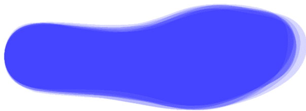
Figure 2. Superimposed treads of 8 shoe lasts of size 38 from different shoe brands (right).
