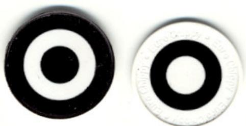
*Fig. 3: Two types of flat ring-shaped markers are used for TERGOSKOP analysis*
