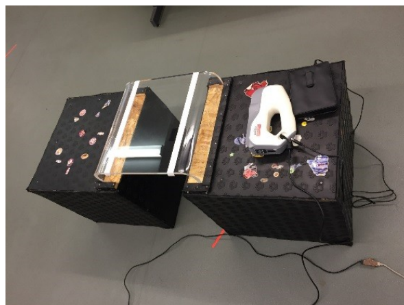
Figure 1: The Perspex platform on the custom built stand and the Artec Eva hand held scanner.
